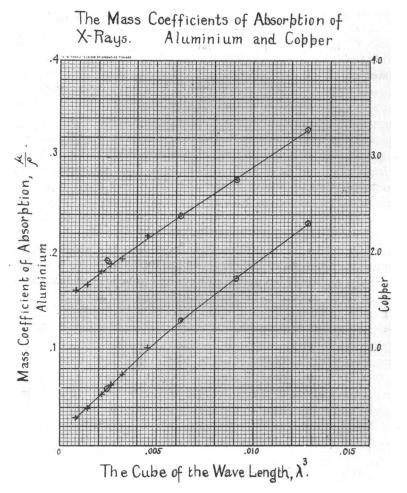
with wave-length, copper should be used for estimating the wave-length of short rays, whereas aluminium is better for longer ones.
